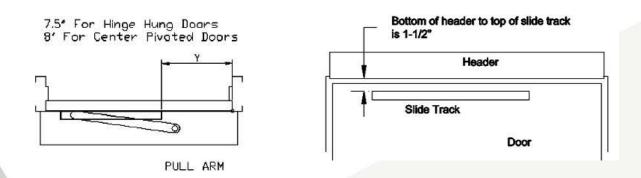
To install the pull arm, and allow proper preload the operator must be powered to the fully open position.
