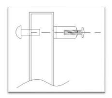
When attaching the header to the hollow metal door frame, ensure there are 5 attaching screws spaced equally apart. They should be #12 sheet metal type screws.
