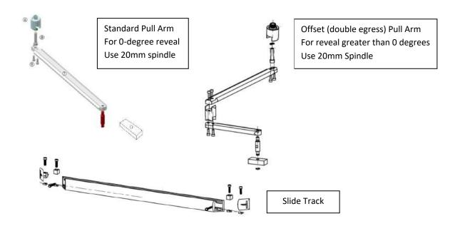
Install the slide track assembly at the pull side of the door at the proper location from the hinge end of the door as shown below:
