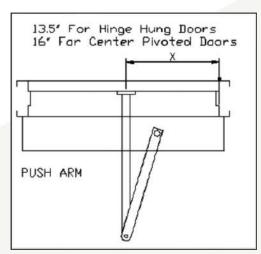
Attach the secondary arm mounting bracket to the door. The centerline of the bracket should be at 13-1/2" in from the inside face of the hinge jamb when using butt hinges on the door, and 16" when using a center pivoted door.
