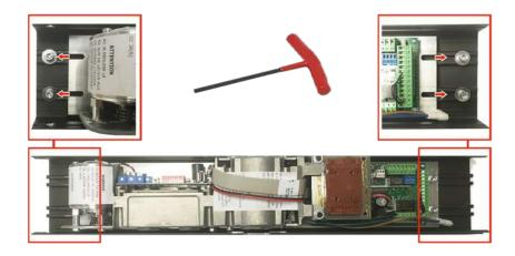
2 Drive plate removed by shifting to the left and lifting the drive plate off the locating screw.
